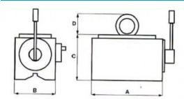
Magnetic lifters are suitable for lifting bars, rounds, sheets, moulds, beams or other pieces of iron. Being made with permanent magnets, they represent the maximum in the safety of lifting, as they do not detach the piece until after the lever has been operated. They have the advantage of being able to move the pieces quickly and avoiding slinging with ropes or chains. Please refer to our instruction manual.
